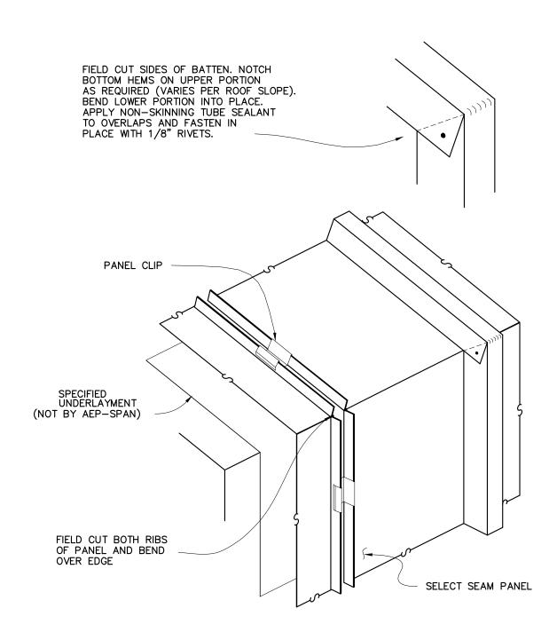
DESIGN CAUTION: TURNING PANELS DOWN FOR FASCIA MAY ESTABLISH UNWANTED POINT OF PANEL FIXITY.
